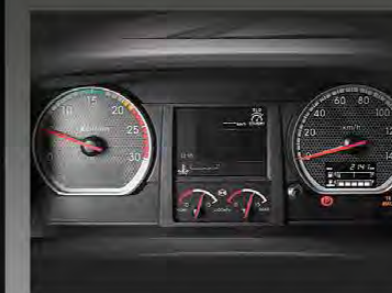
Instrument Meter with Multi-information Display
