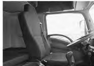
Air Suspension Seat with Integrated Seatbelt
