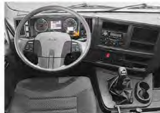
Semi-round Functionally Zoned Instrument Panel
