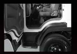
**Easy Egress and Ingress** The built-in step board and steel vertical long grip is designed to provide convenience and safer ingress and egress.
