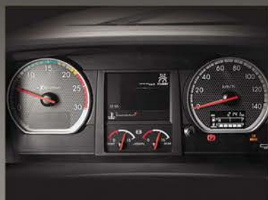
Instrument Meter with Multi-information Display
