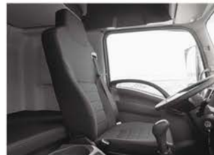
Air Suspension Seat with Integrated Seatbelt
