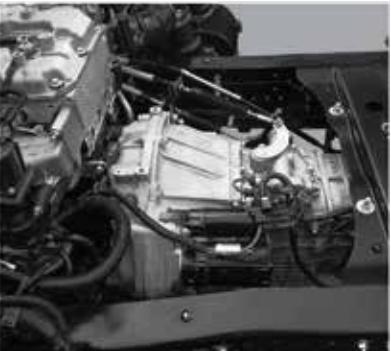
Transmission Comes with either 5-speed or 6-speed MT/AMT.
